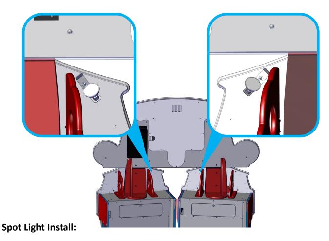
The spot light power wiring for the spot lights are located at each side of the marquee's supports. Cut the tie strap and attach them to the spot lights. The harness length determines which spot light it will plug into. All connections are the same. Two of the harnesses are not used on two cabinet installs.
