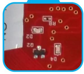
D4- (Brain board), indicates the board is powered and operating.
