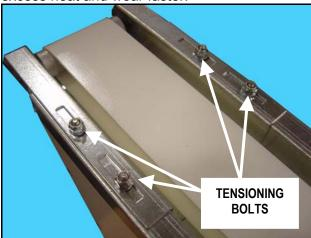
Figure 9 Conveyor Adjustment
