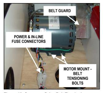
Figure 12 Conveyor Drive Belt Tensioning
