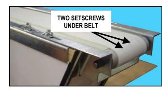
Figure 10 Belt Removal - Exit End
