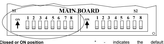
X – Closed or ON position O – Open or OFF position
