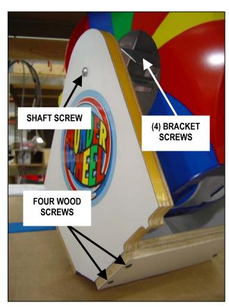
Figure 13 Wheel Disassembly
