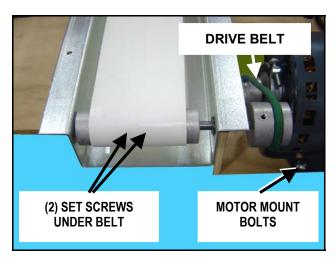
Figure 11 Belt Removal - Drive End
