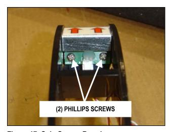
Figure 17 Coin Sensor Board
