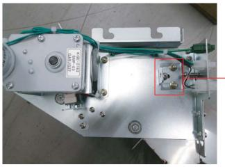
(2) Loosen ③ the bolts and nuts of belt adjustment BKT of FRA to move.
