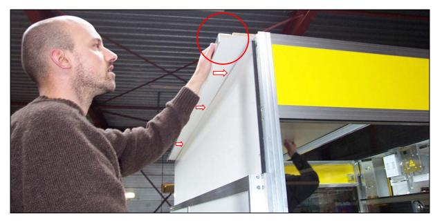
• Slide the front roof-panel into the crane until it lies in the right position.
