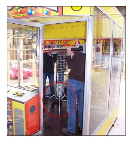
• Remove all the red spanwires from the gantry.
