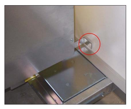
• Put the floor plates in the crane. Start with the largest plate. Make sure that the u-shaped hole is at the back. Put the plate first in its place at the front side and let the plate fall down at the backside (see photo below).
