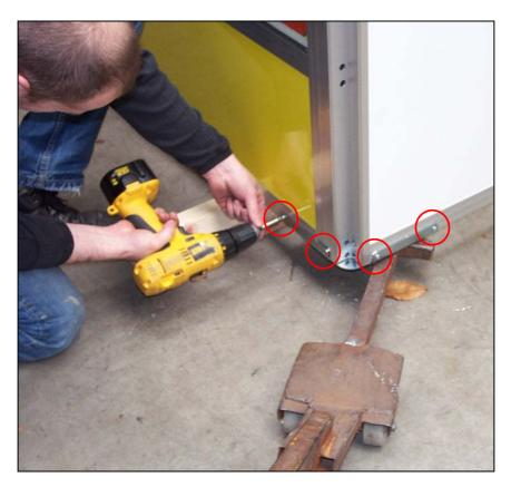
Screw the wheelblocks on to the crane as follows:
