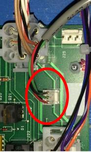
\*\*Note \*\* Attach the upper braces first using 1/4-20 x 1 1/2" bolt and 1/4-20 keep nut. Then side the bracket for the cheat sensor on the bolt and attach with 1/4-20 nylock nut. The wire harness attaches to the upper brace with a tie wrap, down the right side to the front of the cage, down the cage front and into the wire access hole shown in step 9b. It connects to the main board shown.
