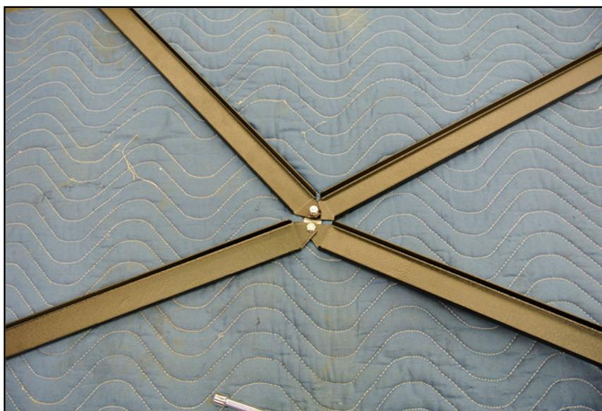
Repeat for the other Pem stud on bracket. Invert the assembly and mount to the four corners of the top of upper frame of the game (2 persons are recommended to perform this part) using ¼-20x3/4” carriage bolts (2) on front of game (see below),
