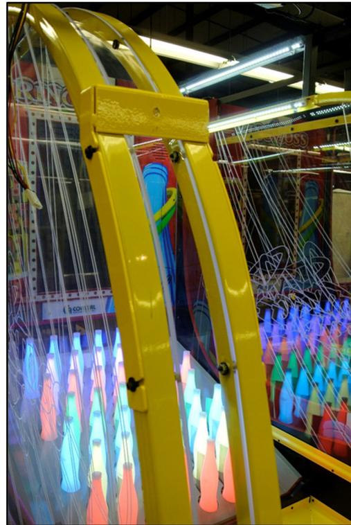
Place one end of bonus sign pole (the end without the holes to pass bolts) over the nub of the boat board (see picture), and secure it to the post holder bracket with a 1/4-20x2 1/2 carriage bolt, using a nut.
