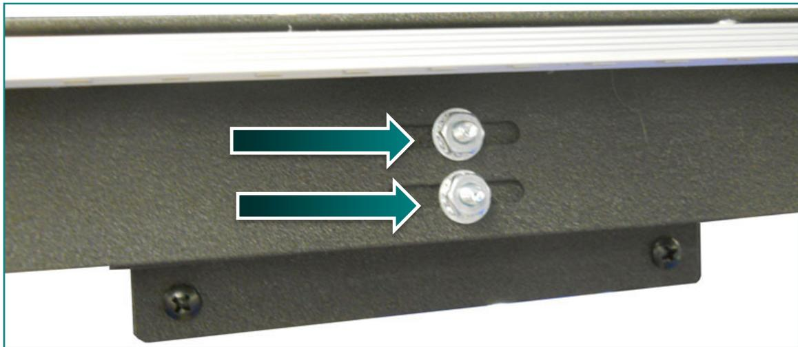
3. Once you have the camera aligned left-to-right and have tightened the nuts back up, you can loosen the screws on the sides of the camera mount to adjust the angle of the camera (green arrows are pointing to the screws):
