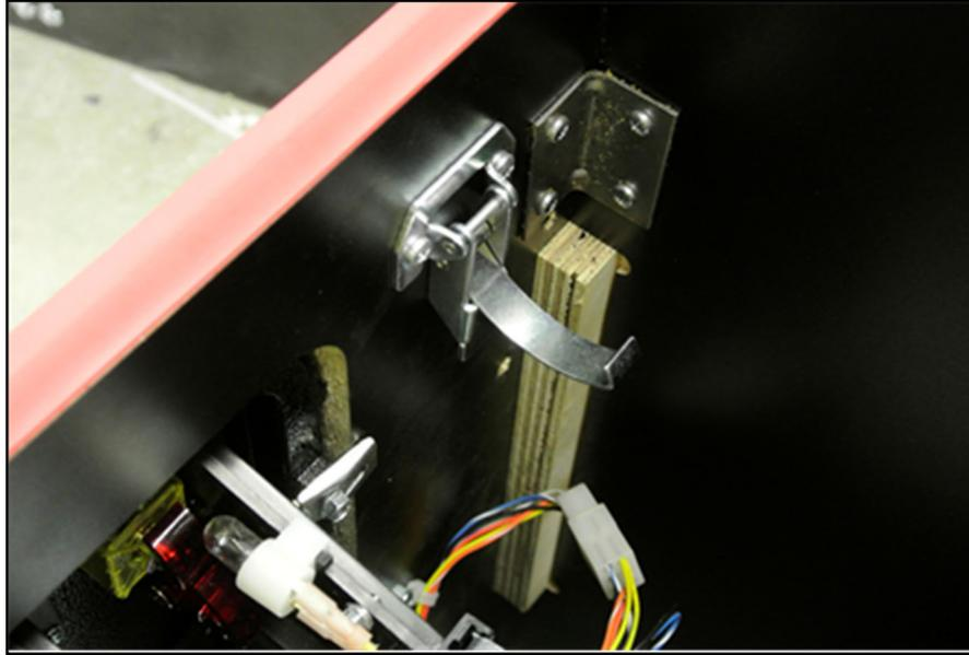
Once released, lift the console lid to open. The wire harness connecting the front console to the main body has multiple connections. The connectors for optical sensors are labeled A, and B. The connectors are such that no accidental mismatching should occur. Power is run through a separate hole in the console.
