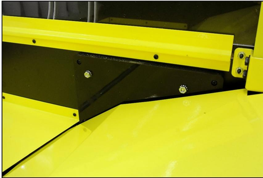
A third bolt (1/4-20x2 1/2") goes from right to left underneath the board with the foul line graphics. Next, the post holder bracket is mounted over the two inside arches using 8-32 x 2" screws (picture-13).
