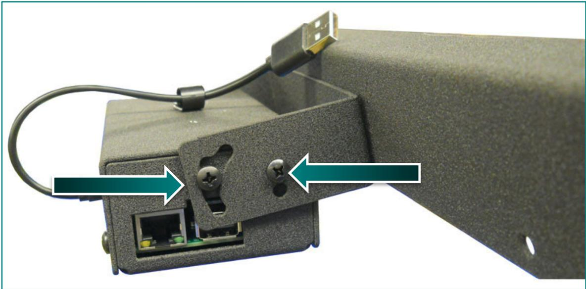
4. There are two screws on either side of the camera mount. Loosen the screws as little as possible so that the angle of the mount can be adjusted and stay in place once you let go of the mount.
